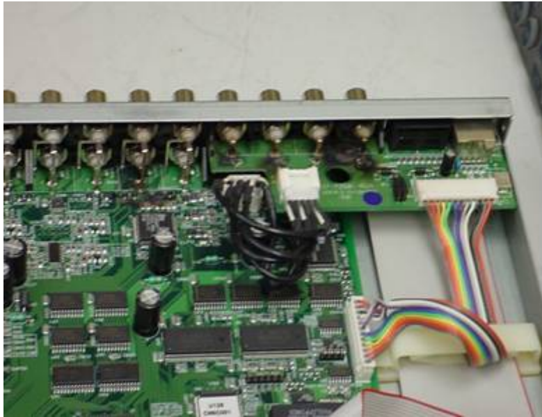
Photos 4: Burn Marks on Multiplexer Inputs
